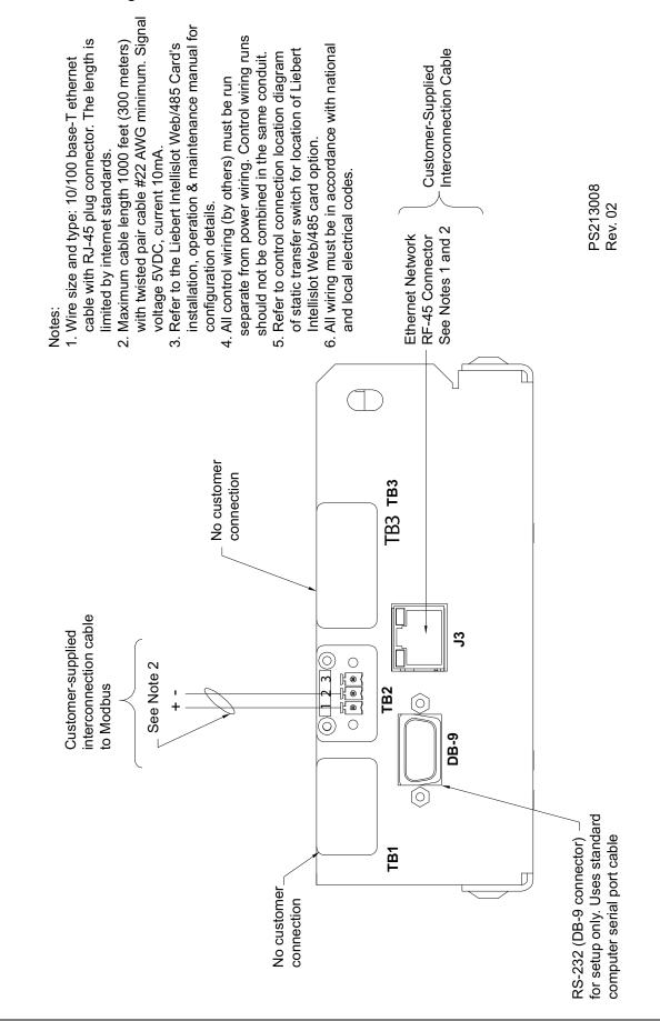
Figure 27 Control wiring for the Liebert IntelliSlot SNMP/Web/Modbus 485 card
